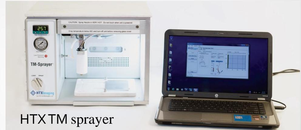
To control the amount of matrix coated onto the tissue sections we used an automatic sprayer as a better way to compare **AP (760 torr)** with **IP ( $10^{-2}$  Torr)**
